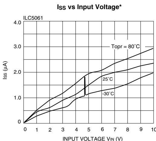
\* A spike of 1/2 to 1 $\mu A$  may appear as  $V_{IN}$  crosses  $V_{DTR}$  or  $V_{DF}$
