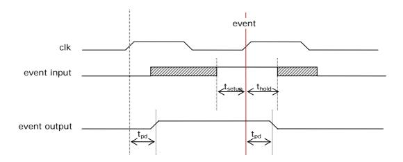
The parameters  $t_{\text{setup}}$ ,  $t_{\text{hold}}$  and  $t_{\text{pd}}$  are technology dependent and must be determined according to the chosen technology.
