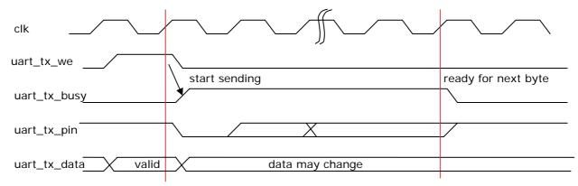
The transmitter path stores the incoming byte in the shift register by means of the uart\_tx\_we signal and starts the transmitting activity. uart\_tx\_busy goes high also and remains high until the data is sent.
