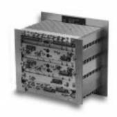
This synthesizer is a custom, iterative indirect synthesis design. It offers fine resolution and low phase noise and spurious over 1 GHz bandwidth in S-Band. Developed prior to the advent of DDS technology, the unit is an example of a complex, highly integrated
