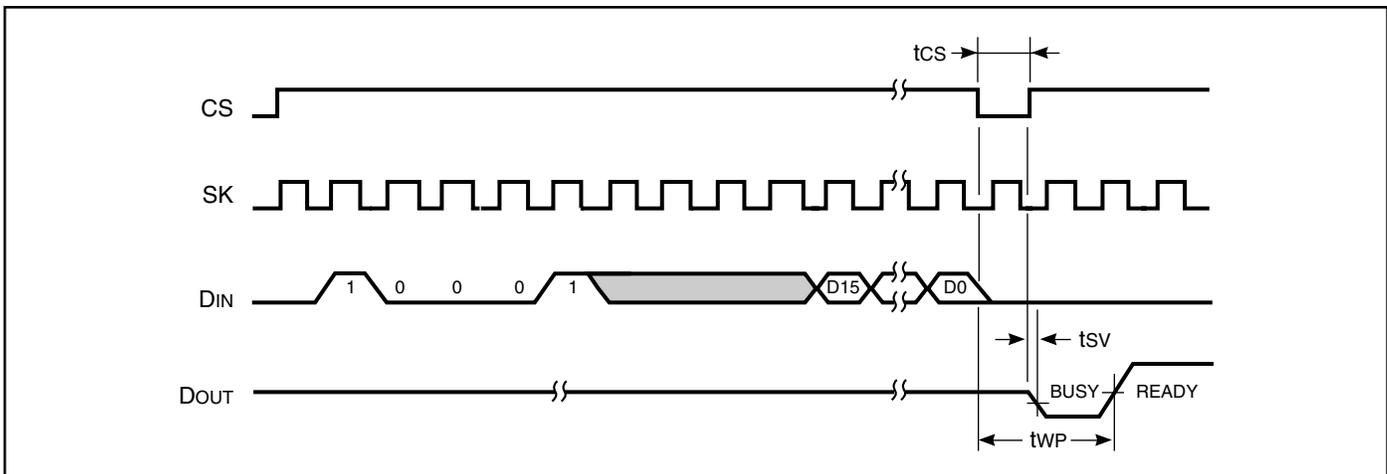
**FIGURE 7. WRITE DISABLE (WDS) CYCLE TIMING**
