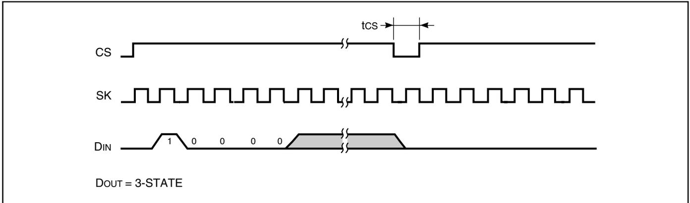
**FIGURE 8. ERASE (REGISTER ERASE) CYCLE TIMING**
