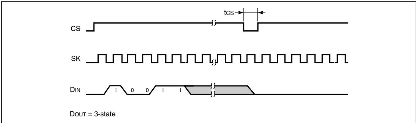
FIGURE 5. WRITE (WRITE) CYCLE TIMING
