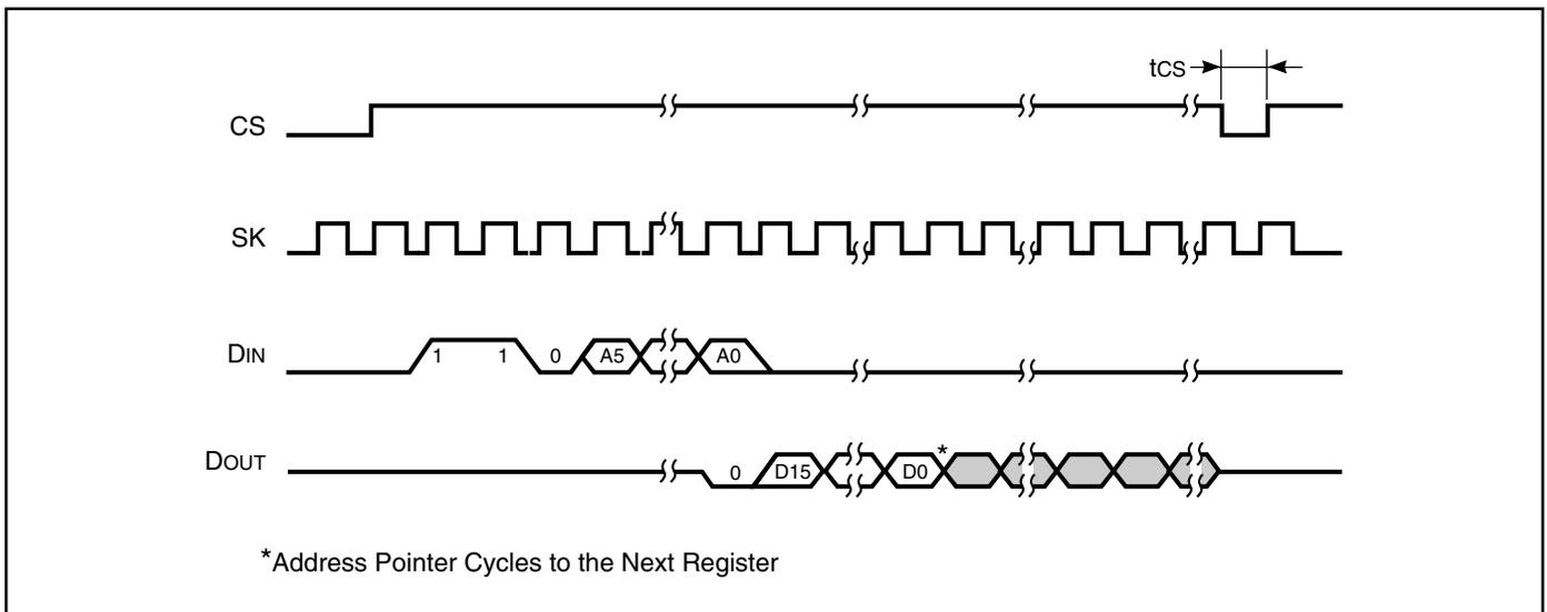
FIGURE 4. SYNCHRONOUS DATA TIMING
