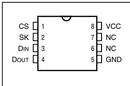
**PIN CONFIGURATION****8-Pin JEDEC Small Outline "G"**
