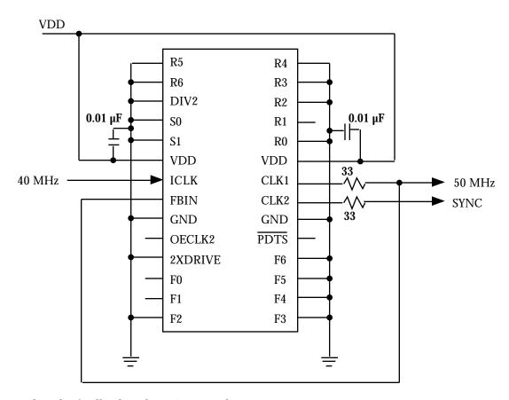
Note that the feedback is done AFTER the series termination resistor.
