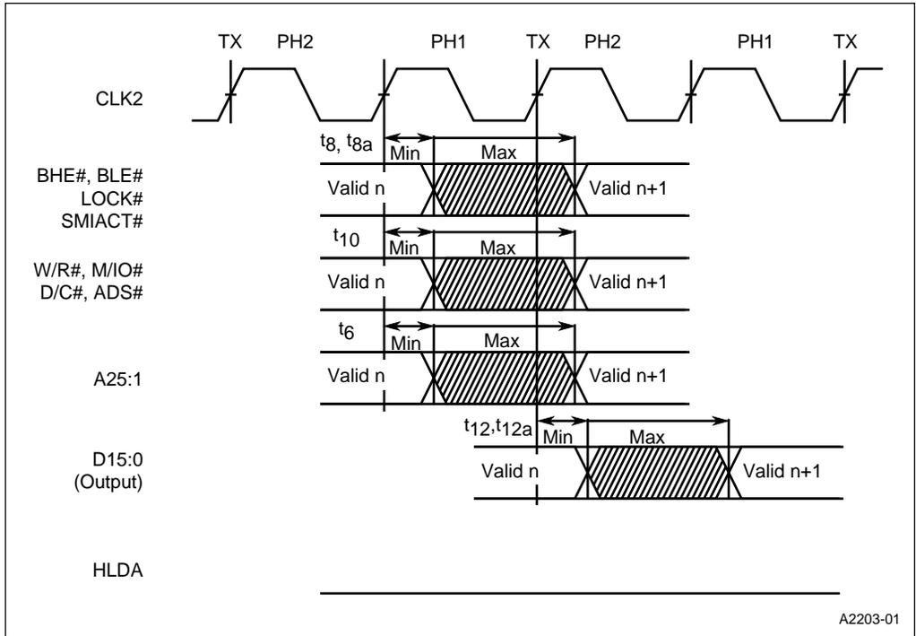
Figure 7. AC Timing Waveforms — Output Valid Delay Timing
