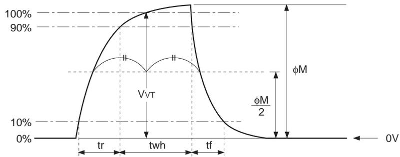
(2) Vertical transfer clock waveform
