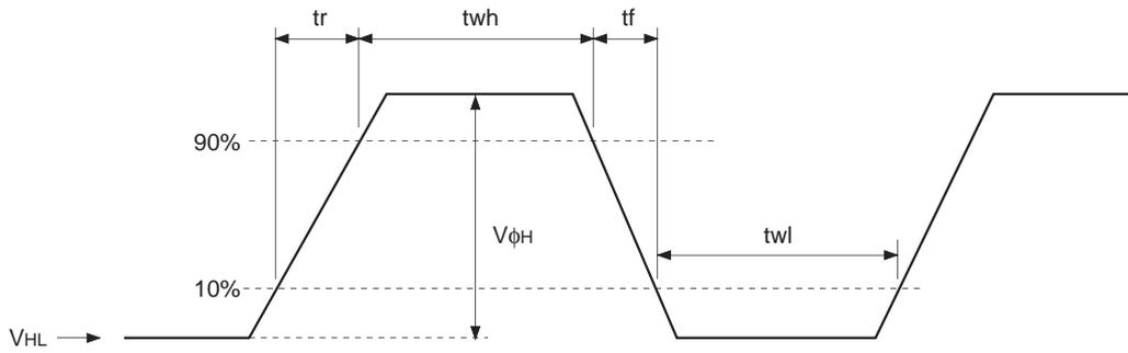
**(4) Reset gate clock waveform**
