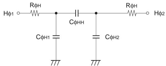
**Horizontal transfer clock equivalent circuit**
