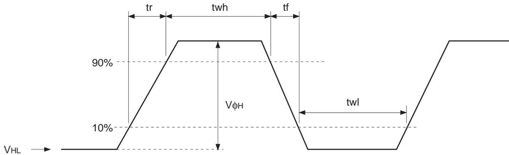
**(4) Reset gate clock waveform**
