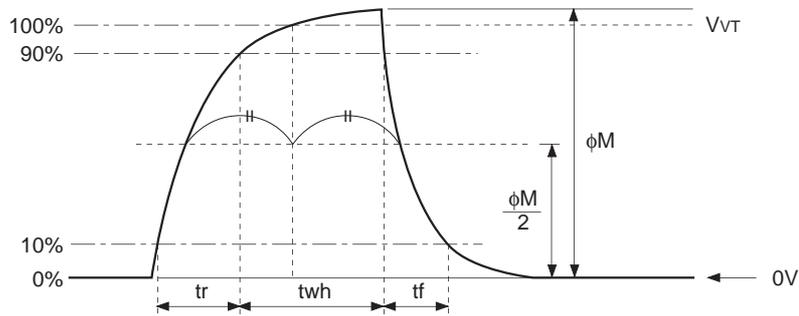
(2) Vertical transfer clock waveform
