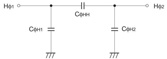
**Horizontal transfer clock equivalent circuit**
