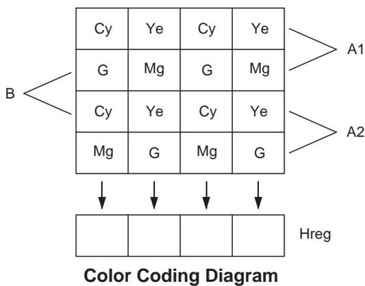
As shown in the left figure, fields are read out. The charge is mixed by pairs such as A1 and A2 in the A field. (pairs such as B in the B field)
