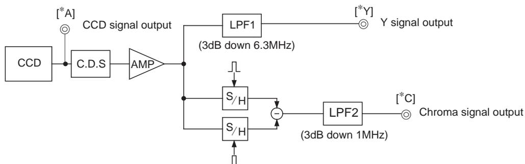
**Note)** Adjust the amplifier gain so that the gain between [\*A] and [\*Y], and between [\*A] and [\*C] equals 1.
