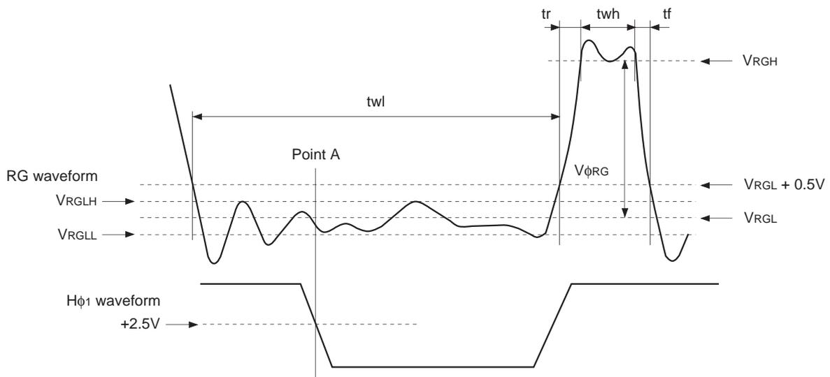
$V_{RGLH}$  is the maximum value and  $V_{RGLL}$  is the minimum value of the coupling waveform during the period from Point A in the above diagram until the rising edge of RG. In addition,  $V_{RGL}$  is the average value of  $V_{RGLH}$  and  $V_{RGLL}$ .
