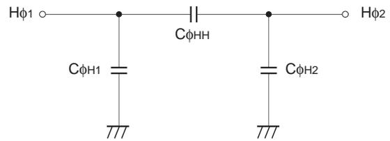
**Horizontal transfer clock equivalent circuit**
