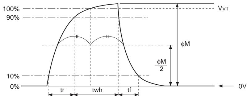
(2) Vertical transfer clock waveform
