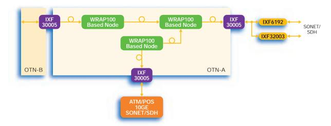
The Intel® IXF30005 may be operated as Intra Domain Interface (IaDI) and Inter Domain Interface (IrDI) within an OTN according to G.709, acting as a gateway between two OTNs or as a network node within an OTN. Because of the various types of framing it supports, the IXF30005 may also act as a gateway between existing IXF30001-based network and an G.709 compliant OTN.
