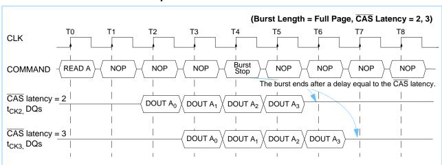
If a Burst Stop Command is issued during a full page burst write operation, then any residual data from the burst write cycle will be ignored. Data that is presented on the DQ pins before the Burst Stop Command is registered will be written to the memory.
