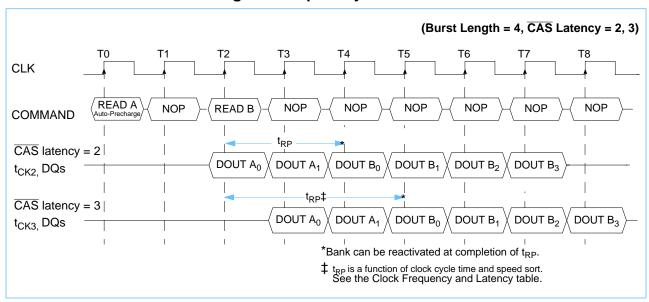
If interrupting a Read Command with auto-precharge with a Write Command, DQM must be used to avoid DQ contention.
