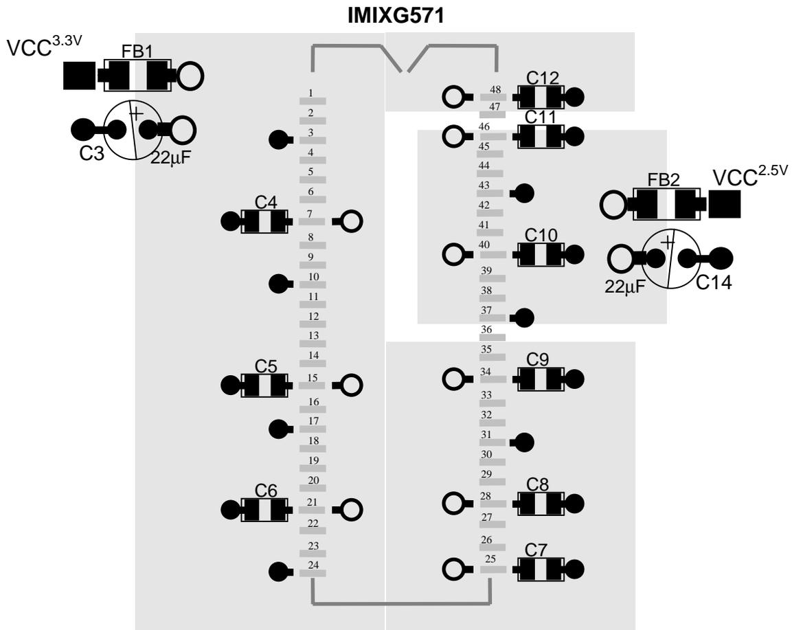
This is only a layout recommendation for best performance and lower EMI. The designer may choose a different approach but C4, C5, C6, C7, C8, C9, C10, C11 and C12 (all are 0.1μf) should always be used and placed close to their VDD pins.
