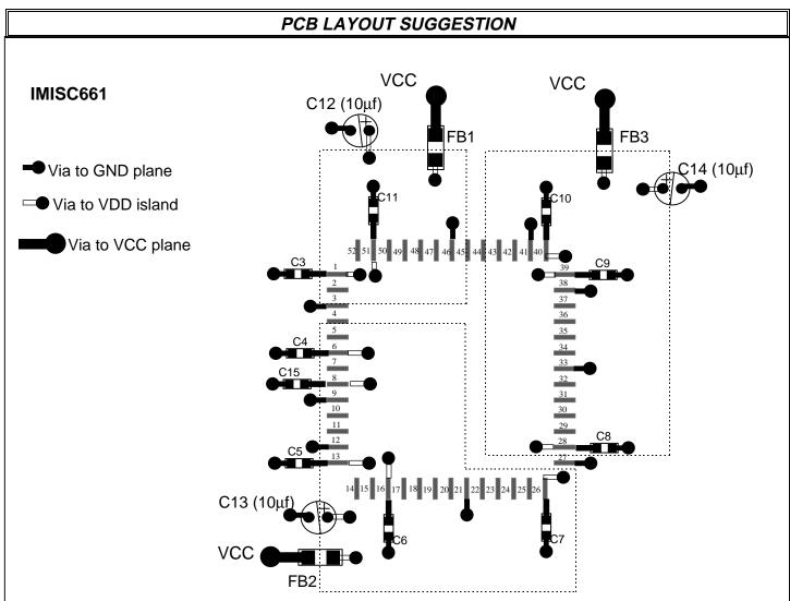
This is only a layout suggestion for best performance and lower EMI. The designer may choose a different approach such as using VDD traces instead of islands (dashed areas). Also, the designer may choose to use less than three beads. Regardless of which way the layout is implemented, Bypass caps: C3, C4, C5, C6, C7, C8, C9, C10, C11 and C15 (all  $0.1\,\mu F$ ) should always be used and placed as close to their VDD pins as possible.
