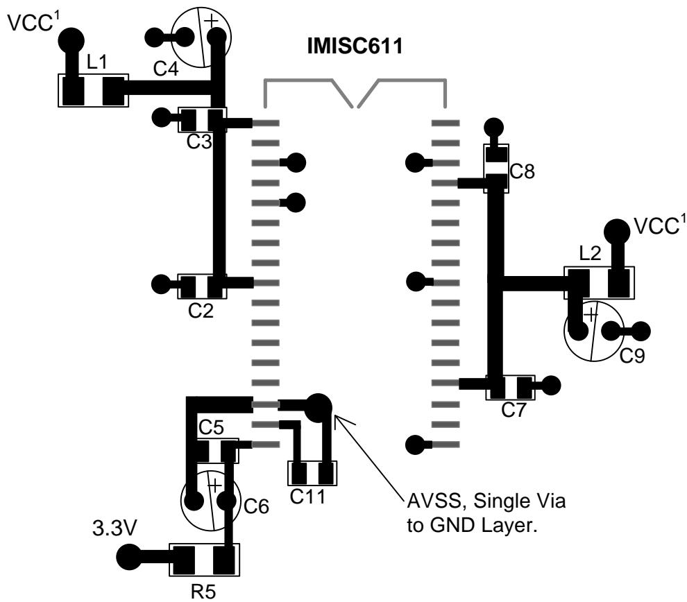
This is only a layout suggestion for best performance and lower EMI. The user may choose a different approach but C2, C3, C5, C7, and C8 should be always be used and placed close to their VDD pins.
