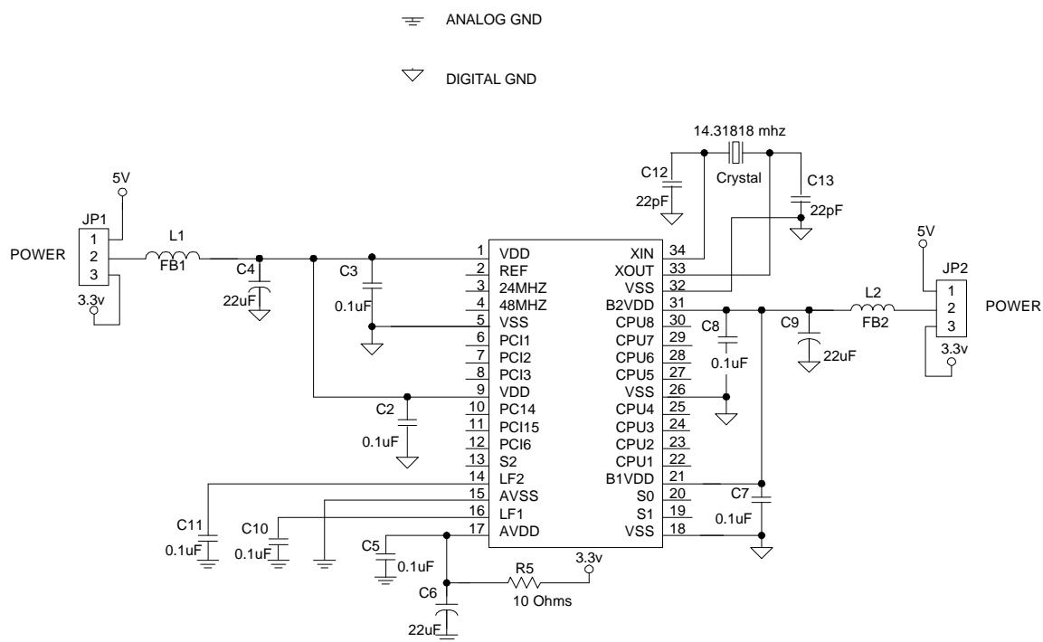
NOTE 1: PIN21, B1VDD MAY HAVE ITS OWN POWER (INDEPENDENT OF B2VDD, PIN 31)
