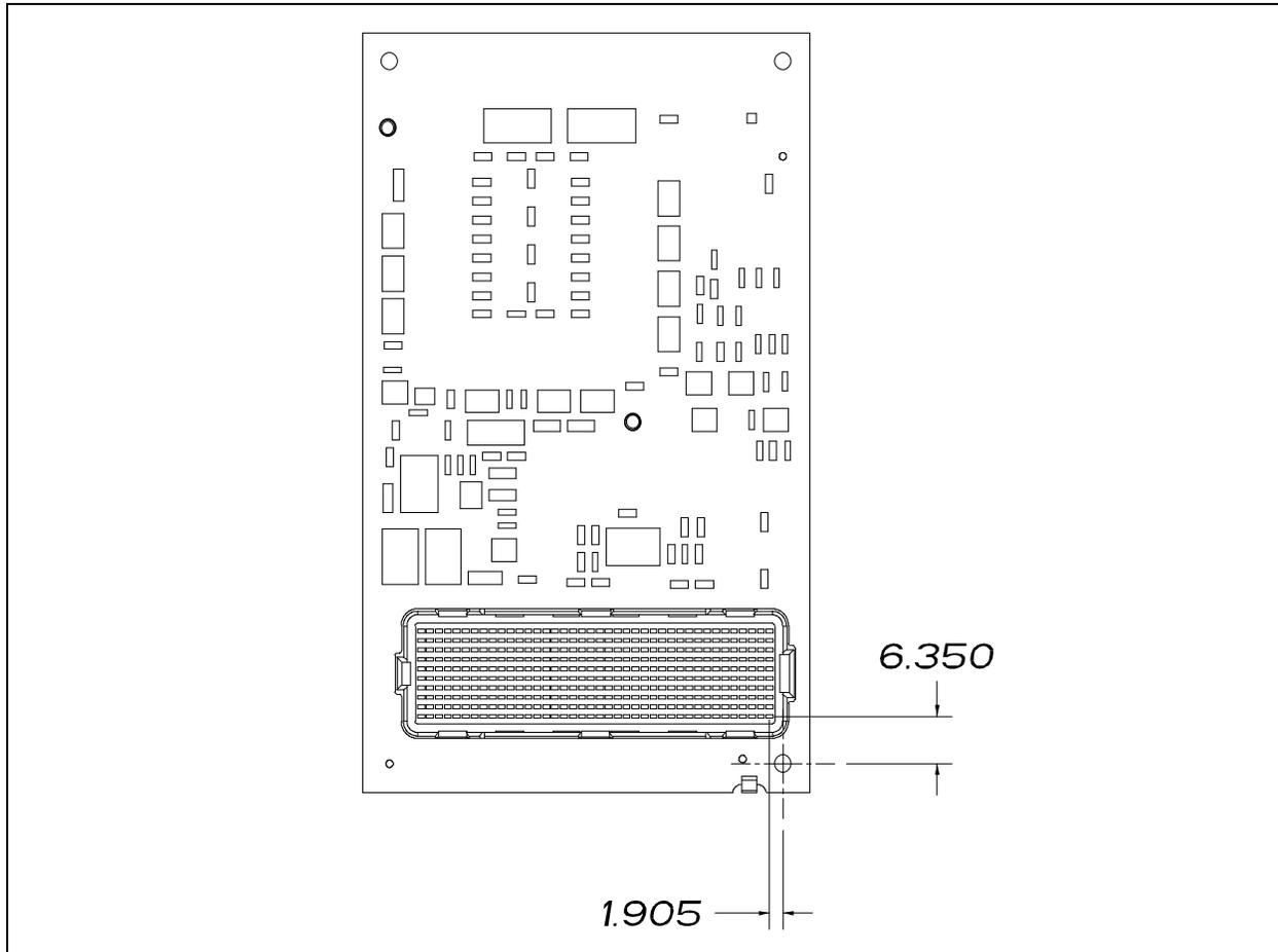
Figure 11. Board Dimensions with 400-Pin Connector- Pin 1 Orientation
