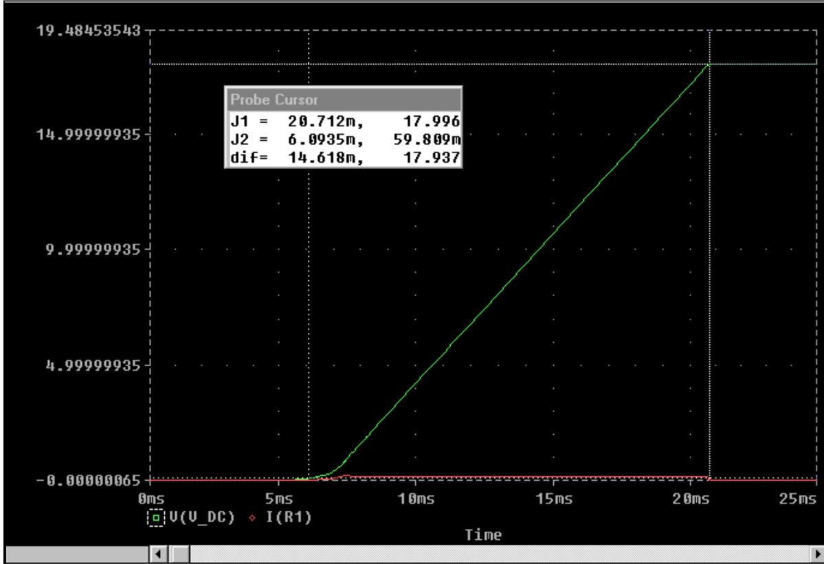
Figure 9. Spice Simulation Using In-rush Protection (Example ONLY)
