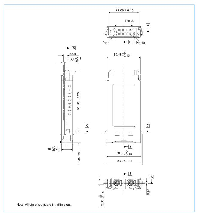
Two optical receptacles are at the end of the module. They are spaced 12.7mm apart to accept a standard duplex SC connector.
