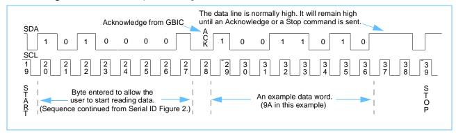
**Serial ID Figure 4** Critical Timings for GBIC-1063NS, GBIC-1063NS-LW, GBIC-1250NS, and GBIC-1250NS-LW Parameters are defined in Serial ID Timing Specifications on page 21.
