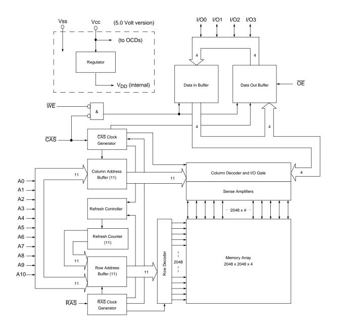
IBM0117400 IBM0117400M IBM0117400B IBM0117400P **4M x 4 11/11 DRAM**  IEM
