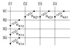
All the resistors are  $330k\Omega$ . The resistor option functions and the default specifications (without option resistors) are listed below.
