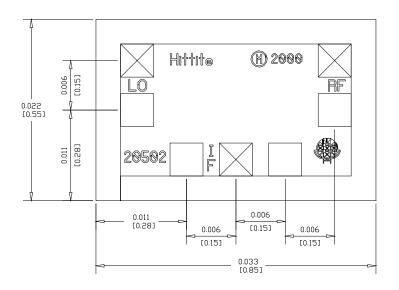
Backside of chip is ground. Connections are not required for unlabeled bondpads.
