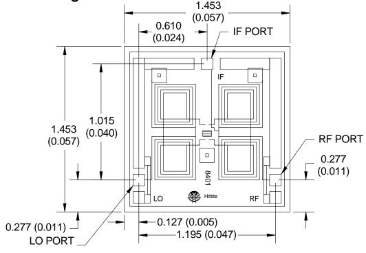
DIE THICKNESS IS 0.100 (0.004), BACKSIDE IS GROUND BOND PADS ARE 0.100 (0.004) SQUARE ALL DIMENSION IN MILLIMETERS (INCHES) ALL TOLERANCES ARE ± 0.025 (±0.001) BOND PAD METALLIZATION: GOLD BACKSIDE METALLIZATION: GOLD
