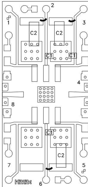
The grounded Co-Planar Wave Guide (G-CPW) PCB input/output transitions allows use of Ground-Signal-Ground (GSG) probes for testing. Suggested probe pitch is 400µm (16 mils). Alternatively, the board can be mounted in a metal housing with 2.4 mm coaxial connectors.
