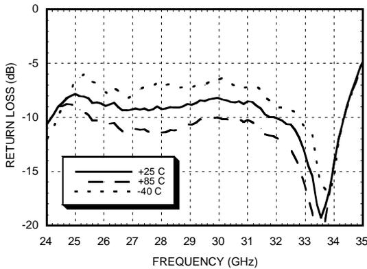
**Output Return Loss vs. Temperature @ Vdd= +6V**
