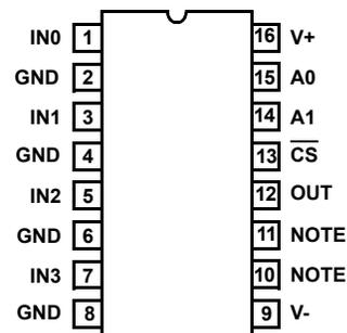
NOTE: These pins must be left floating or connected to ground.
