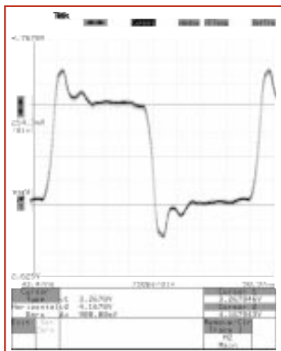
Figure 2: 155.52 MHz PECL oscillator, showing steep rise and fall times and excellent duty cycle. Levels have 900 mv difference between "1" and "0". Overshoots are caused by inductance of socket.
