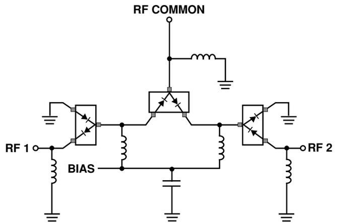
Figure 10. Very High Isolation SPDT Switch, Dual Bias.
