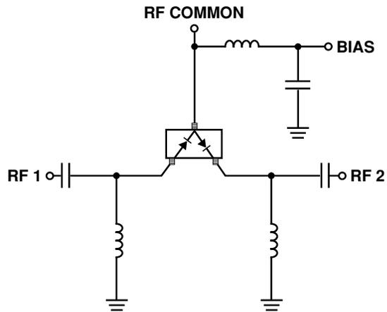
Figure 9. Switch Using Both Positive and Negative Current.
