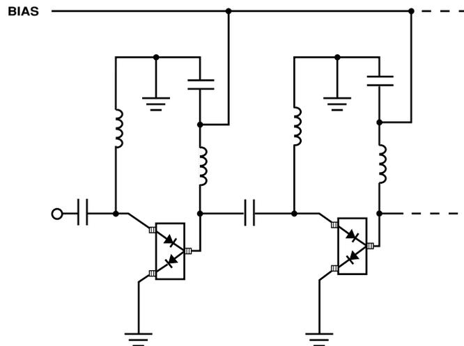
Figure 12. High Isolation SPST Switch
