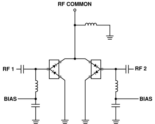
Figure 8. High Isolation SPDT Switch, Dual Bias.
