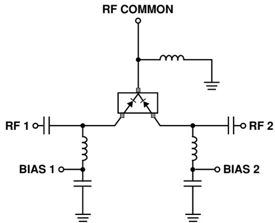
Figure 7. Simple SPDT Switch, Using Only Positive Current.
