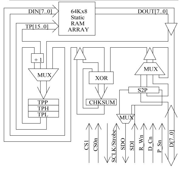
The Table Pointer register keeps the address of SRAM being written to or read from. automatically increment by one with each read/write access, but remains unchanged when writing command or reading checksum.
