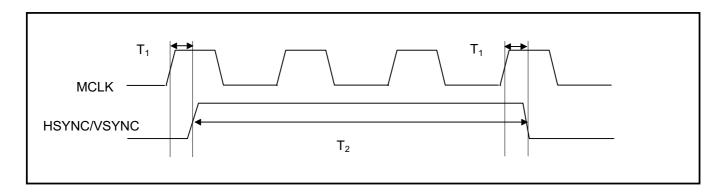
T<sub>1</sub>: MCLK rising to HSYNC/VSYNC valid maximum time: 18ns [output load: 60pF]
