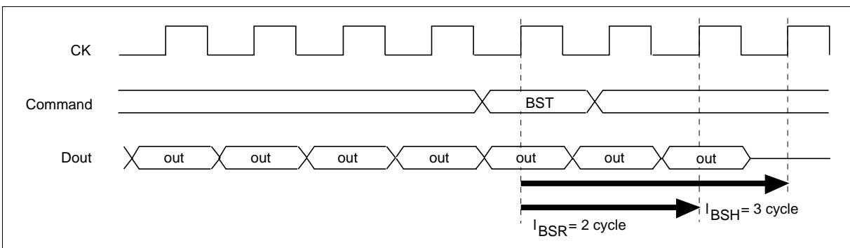
**Burst stop command at burst write:** The burst stop command (BST command) is used to stop data input during a full-page burst write. No data is written in the same clock as the BST command, and in subsequent clocks. In addition, the BST command is only valid during full-page burst mode, and is illegal with burst lengths of 1, 2, 4 and 8. And an interval of  $t_{DPL}$  is required between last data-in and the next precharge command.
