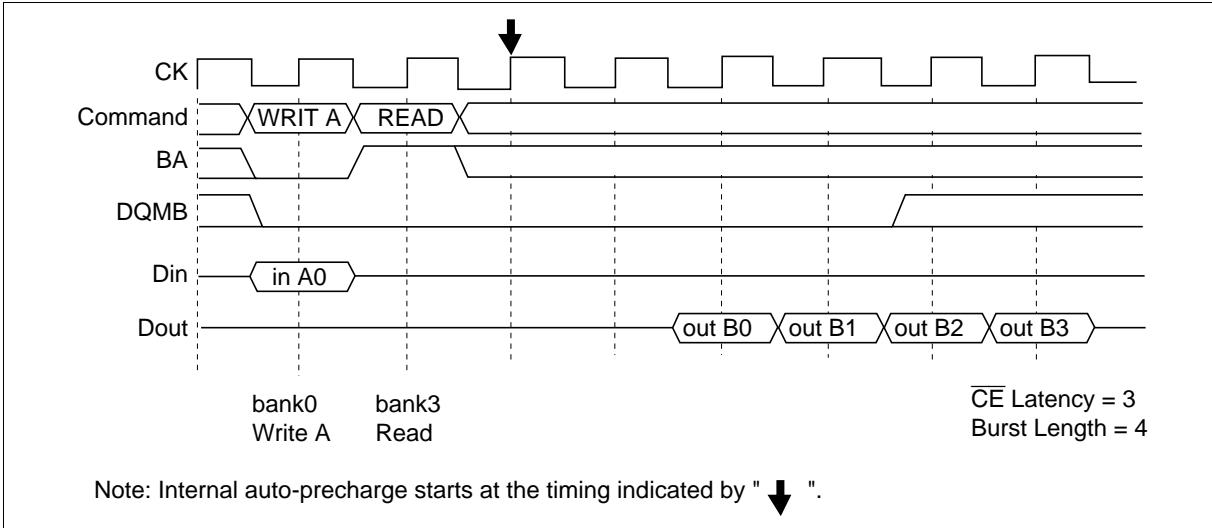
**2. Same bank:** The consecutive read command from write with auto precharge (the same bank) is illegal. It is necessary to separate the two commands with a bank active command.
