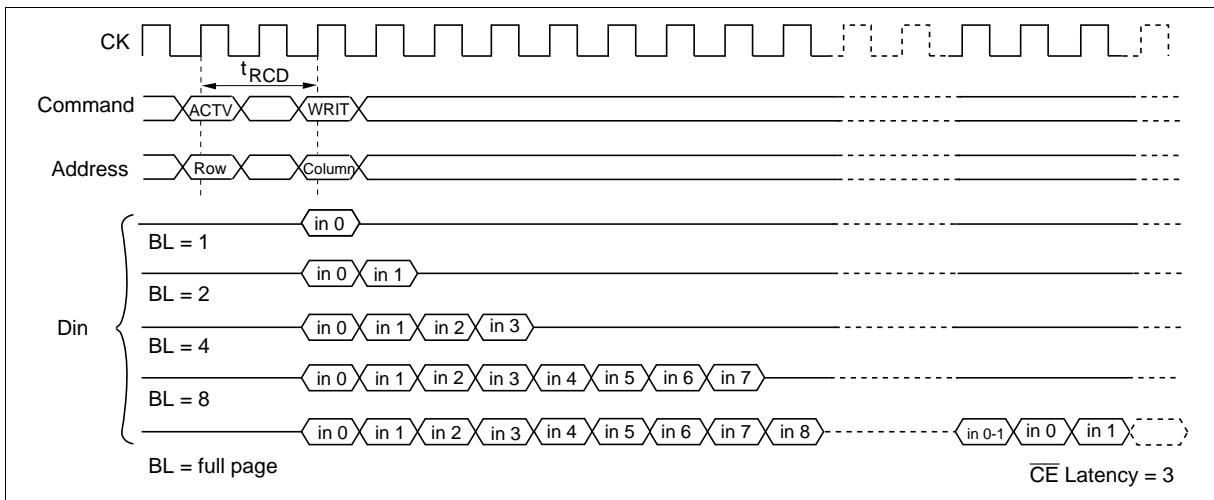
**2. Single write:** A single write operation is enabled by setting OPCODE (A9, A8) to (1, 0). In a single write operation, data is only written to the column address and the bank select address (BA) specified by the write command set cycle without regard to the burst length setting. (The latency of data input is 0 clock).
