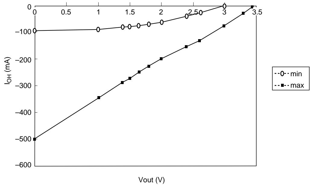
DC Characteristics (Ta = 0 to 65°C, V<sub>CC</sub> = 3.3 V ± 0.3 V, V<sub>SS</sub> = 0 V)
