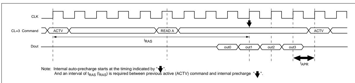
**Write with auto-precharge:** In this operation, since precharge is automatically performed after completing a burst write or single write operation, a precharge command need not be executed after each write operation. The command executed for the same bank after the execution of this command must be the bank active (ACTV) command. In addition, an interval of  $t_{APW}$  is required between the final valid data input and input of next command.
