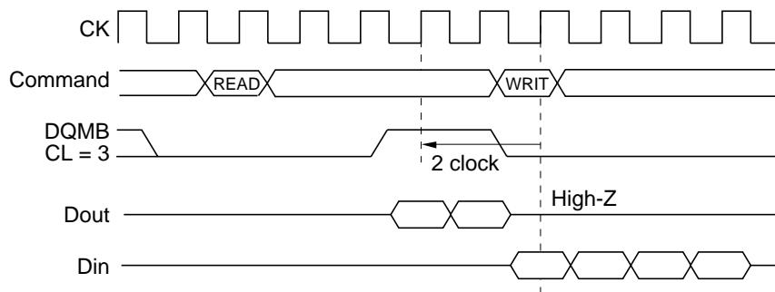
**2. Same bank, different ROW address:** When the ROW address changes, consecutive write commands cannot be executed; it is necessary to separate the two commands with a precharge command and a bank-active command.
