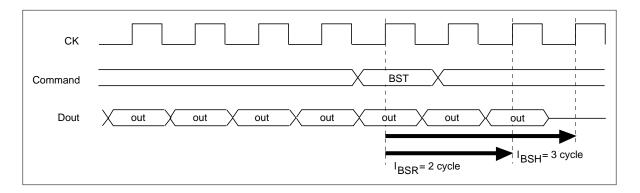
**Burst stop command at burst write:** The burst stop command (BST command) is used to stop data input during a full-page burst write. No data is written in the same cycle as the BST command and in subsequent cycles. In addition, the BST command is only valid during full-page burst mode, and is invalid with burst lengths of 1, 2, 4 and 8. And an interval of  $t_{DPL}$  is required between the BST command and the next precharge command.
