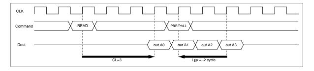
READ to PRECHARGE Command Interval (same bank): To stop output data
