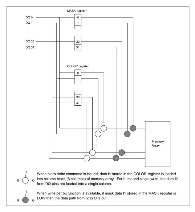
Column address and block write command: For a row of one of two banks activated by ACTV or
