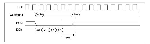
Block Write Command to Precharge Command Interval: The minimum interval between block write command and the following precharge command is  $t_{\text{BWR}}$ .
