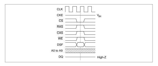
**Ignore command (DESL):** At the CLK rising edge, by setting  $\overline{\text{CS}}$ ; HIGH, any input is ignored.
