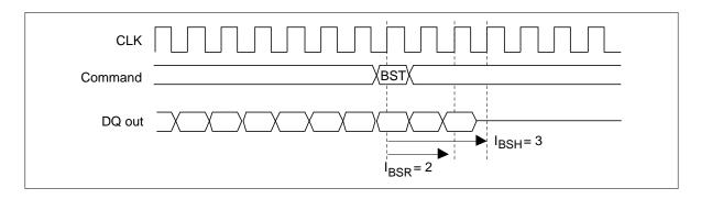
**Burst stop command at burst write:** For full page burst write cycle, when a burst stop command is issued, the write data at that cycle and the following write data input are ignored. The BST command is legitimate only in case full page burst mode, and is illegal for burst length 1, 2, 4 or 8.
