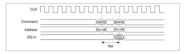
**Special Mode Register Set to Block Write/Write Interval:** The minimum interval between a special mode register set and a block write/write is  $t_{SBW}$ .
