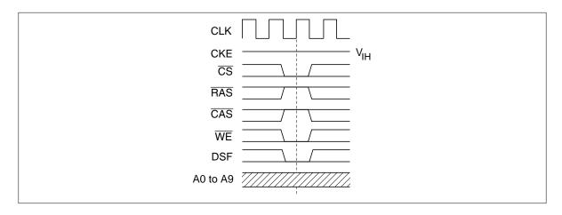
**Auto refresh command (REF):** If both banks are in idle state, at the CLK rising edge, by setting  $\overline{CS}$ ,  $\overline{RAS}$ ,  $\overline{CAS}$ , DSF; LOW,
