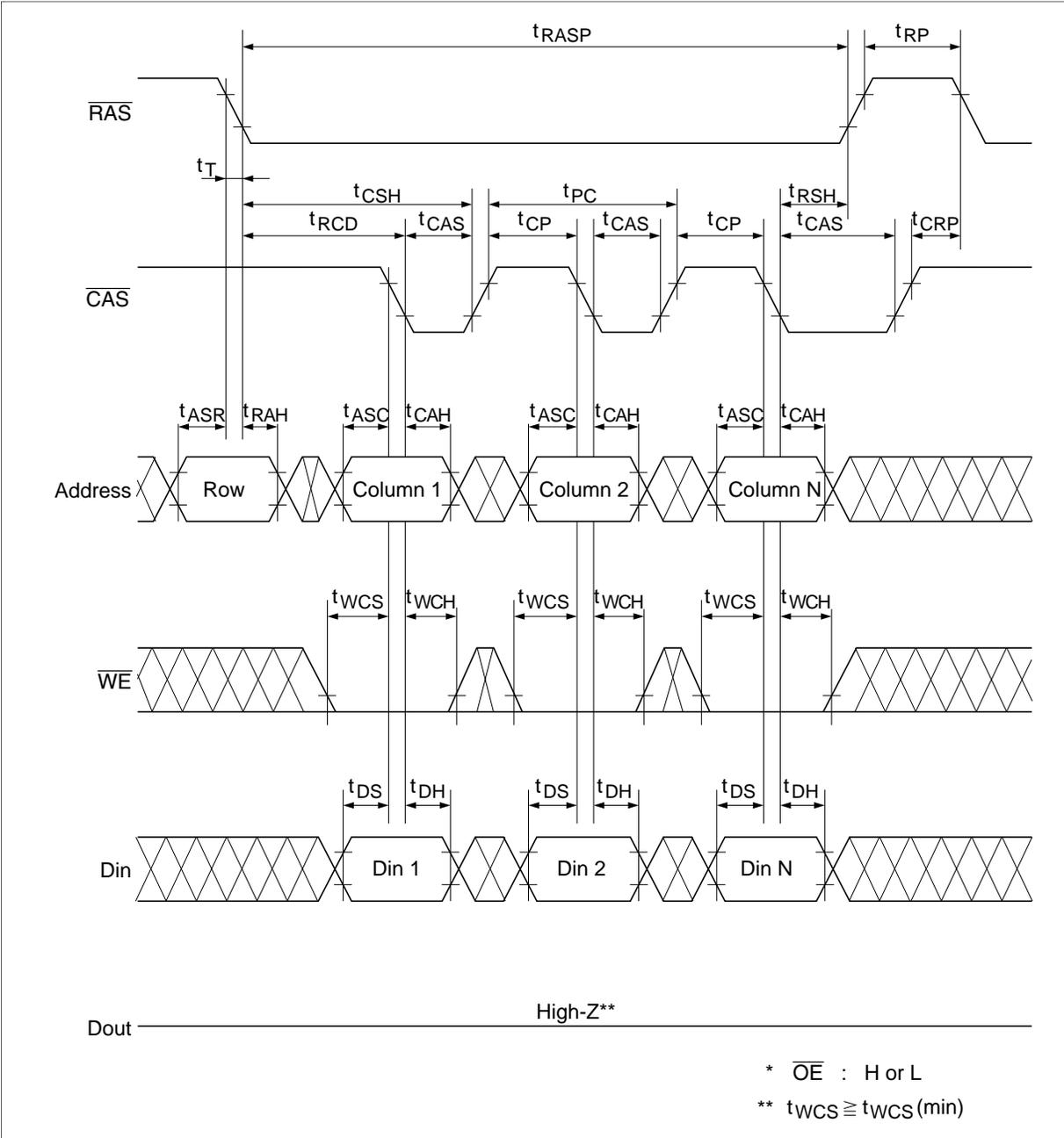
Fast Page Mode Delayed Write Cycle<sup>\*19</sup>
