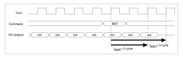
**Burst stop command at burst write:** The burst stop command (BST command) is used to stop data input during a full-page burst write. Data is still written in the same cycle as the BST command, but no data is written in subsequent cycles. In addition, the BST command is only valid during full-page burst mode, and is invalid with burst lengths of 1, 2, 4 and 8. And an interval of  $t_{RWL}$  is required between the BST command and the next precharge command.
