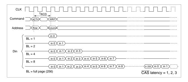
**2. Single write:** A single write operation is enabled by setting OPCODE (A9, A8) to (1, 0). In a single write operation, data is only written to the column address (AY0 to AY7) and the bank select address (A9) specified by the write command set cycle without regard to the burst length setting. (The latency of data input is 0).
