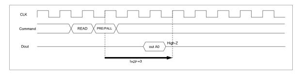
Write command to Precharge command interval (same bank): When the precharge command is executed for the same bank as the write command that preceded it, the minimum interval between the two commands is 1 cycle. However, if the burst write operation is unfinished, the input data must be masked by means of DQMU and DQML for assurance of the cycle defined by  $t_{\rm RWL}$ .
