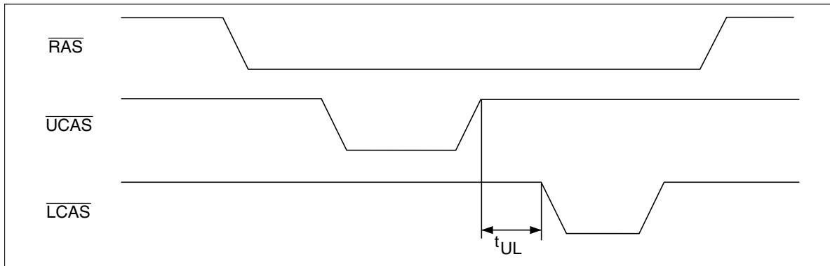
4. Byte control operation by remaining  $\overline{\text{UCAS}}$  or  $\overline{\text{LCAS}}$  high is guaranteed.
