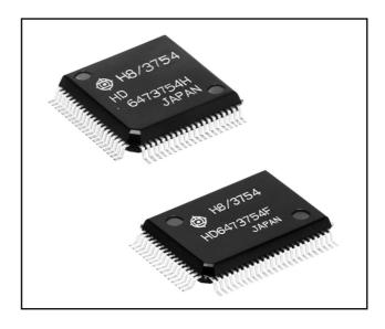
an A/D converter, and I/O ports. Since these microcomputers include high breakdown voltage pins that can directly drive VFD panels, they are particularly suited for use in applications that require VFD.
