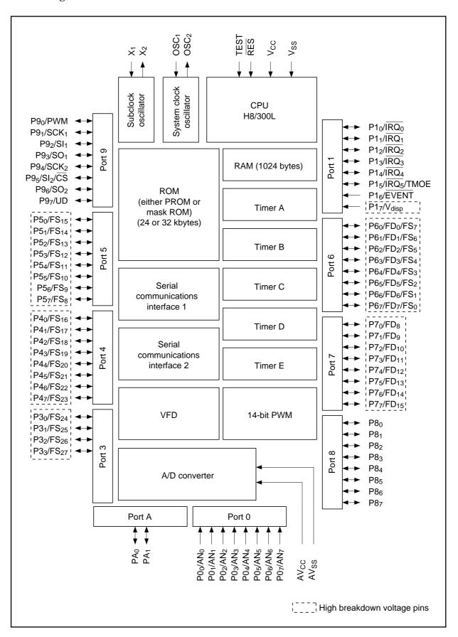
The H8/3814 Series microcomputers are 8-bit single chip microcomputers that can directly drive liquid crystal display (LCD).
