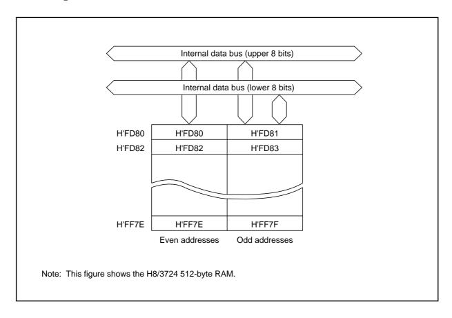
A short absolute addressing mode is provided by the H8/300L Series CPU MOV instruction for rapid access to locations from H'FF00 to H'FFFF. Furthermore, programs can be coded compactly due to the short instruction length. Since RAM locations H'FF00 to H'FF7F can be accessed by this short absolute addressing mode, programs can use this mode to implement high speed data handling.
