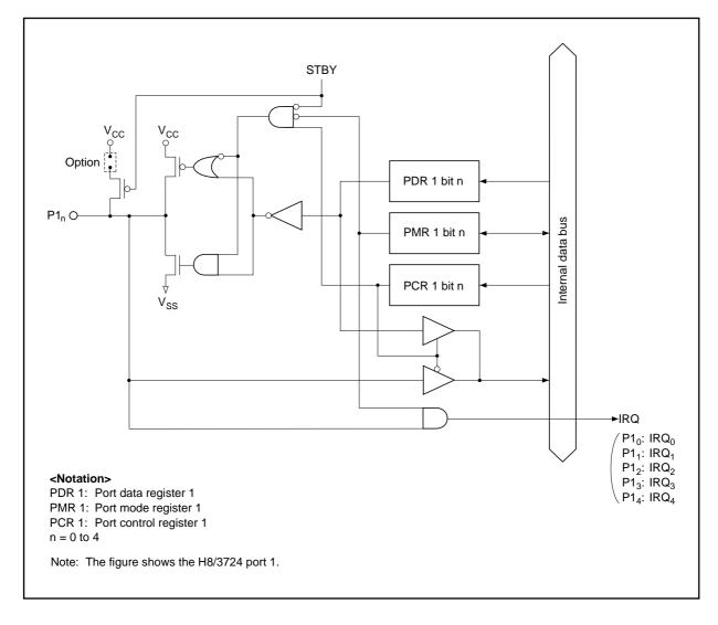
General Purpose I/O Ports with Built-In Pull-Up MOS Transistors: The H8/300L Series general purpose I/O ports are provided with pull-up MOS transistors. In some products, the pull-up MOS transistors can be enabled as a mask option, and in other products, the pull-up MOS transistors can be controlled by application programs.
