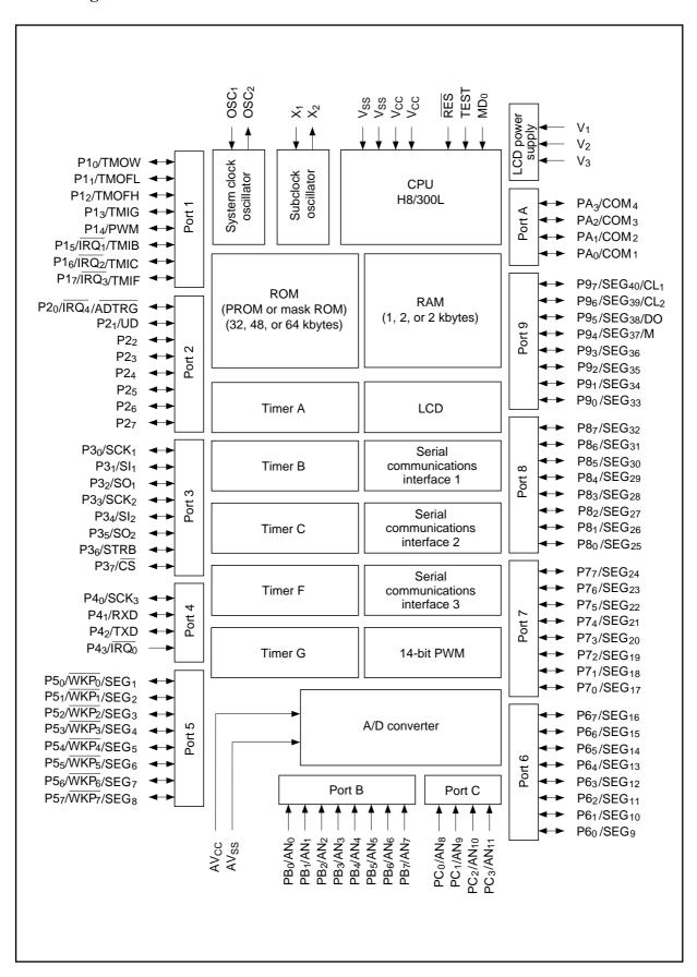
The H8/3877 Series microcomputers are 8-bit single chip microcomputers that can output tones of arbitrary frequencies.
