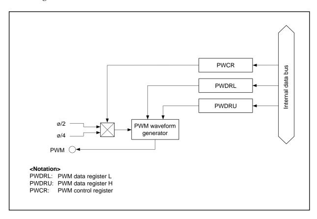
**14-Bit PWM Operation:** The total time  $(T_H)$  of the 64 pulses generated in a single conversion cycle corresponds to the data loaded into the PWM data registers L and H as described by the formula below.
