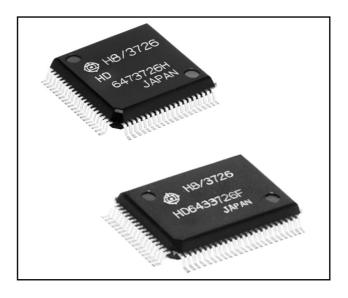
timers, two serial communications interfaces, a 14-bit PWM, an A/D converter, and I/O ports. Since these microcomputers include high breakdown voltage pins that can directly drive VFD panels, they are particularly suited for use in applications that require VFD.
