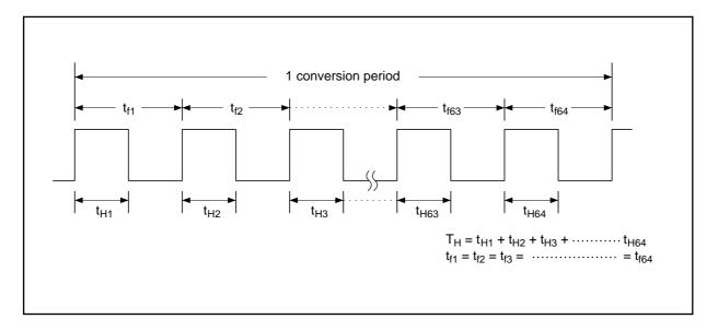
The output will be a high level output (100%) when the data value is between H'3FC0 and H'3FFF. The minimum conversion width pulse is output when the data value is H'0000.
