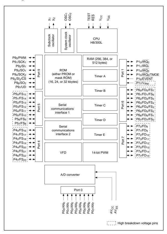
The H8/3724 Series microcomputers are 8-bit single chip microcomputers that can directly drive vacuum fluorescent displays (VFD).
