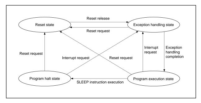
**Reset State:** The H8/300L CPU is reset in this state.
