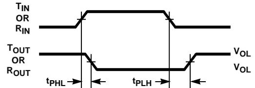
$$\text{AVERAGE PROPAGATION DELAY} = \frac{t_{PHL} + t_{PLH}}{2}$$
