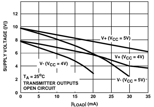
FIGURE 6.  $V_+$ ,  $V_-$  OUTPUT VOLTAGE vs LOAD
