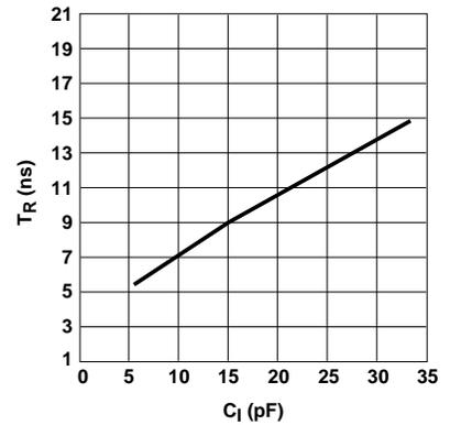
Figure 9. Typical Rise Time vs. Load Capacitance.
