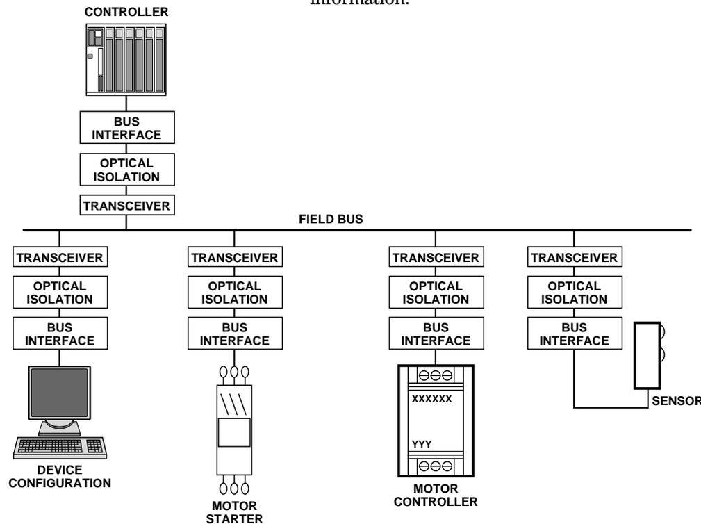
Figure 17. Typical Field Bus Communication Physical Model.
