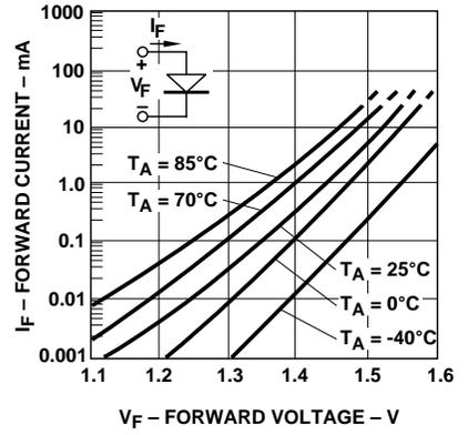
Figure 3. Input diode forward current vs. forward voltage.
