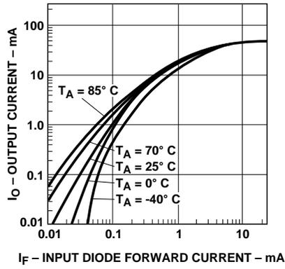
Figure 2. Output current vs. input diode forward current.
