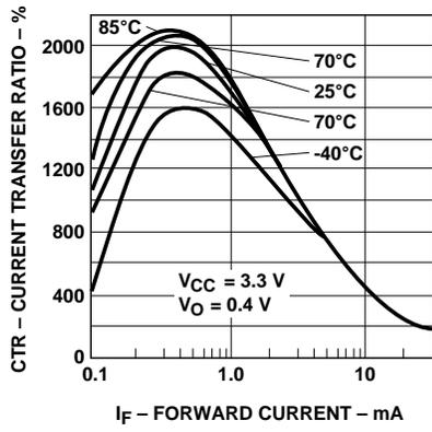
Figure 1. Current transfer ratio vs. forward current.
