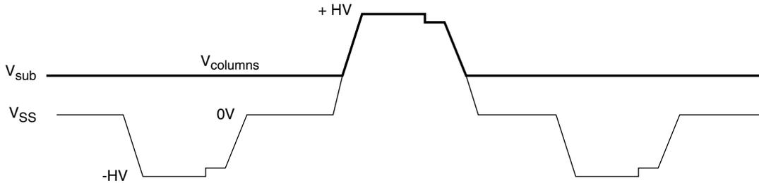
**Note:** In general, when driving the outputs positive,  $V_{sub} = +HV$ . And when driving outputs negative,  $V_{sub}$  equals most positive voltage; e.g. GND or  $>0V$ .
