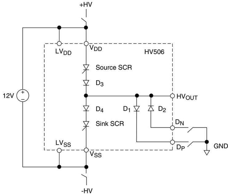
**Note:** The voltage potential between LV<sub>DD</sub>/V<sub>DD</sub> and LV<sub>SS</sub>/V<sub>SS</sub> must not exceed recommended operating conditions of 10.8V - 13.2V (12V typical)
