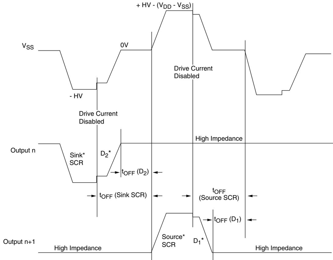
\* Notes internal device handling current flow. Refer to Typical Output Circuit Connections for schematic.
