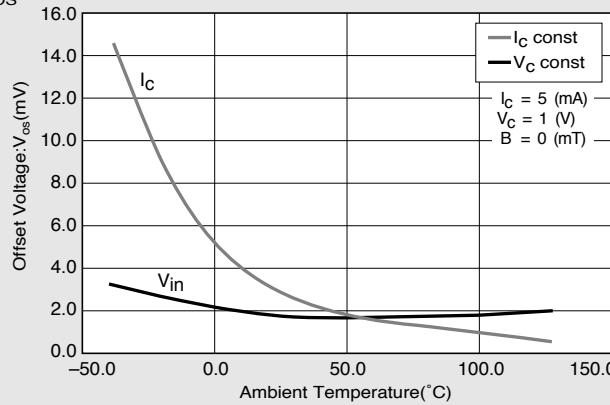
$V_{OS}$ - $V_C$ ,  $V_{OS}$ - $I_C$
