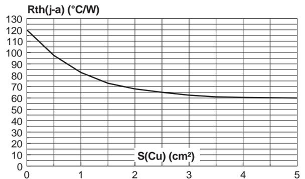
**Note:**  $R_{th}(j-a) = (T_{jMax} - T_{amb}) / P_{Max}$
