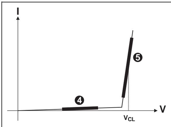
The clamping voltage ( $V_{cl}$ ) is depending on several parameters which are :
