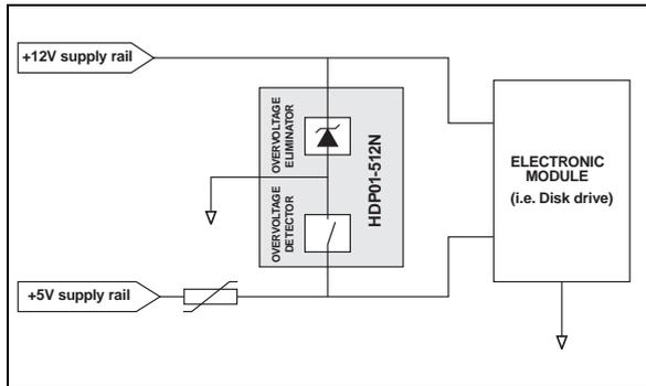
This protection device is able to protect both +5 and +12 Volts power rails against transients and rails inversion.
