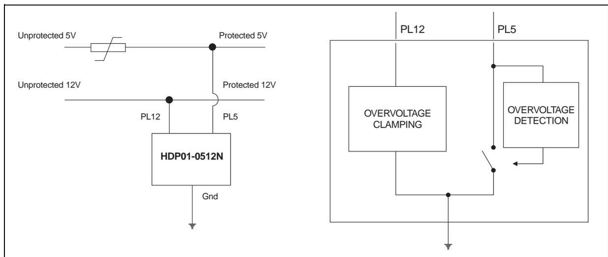
note: The element in series with the 5V line is a resettable device, like Raychem Polyswitch MiniSMD075.
