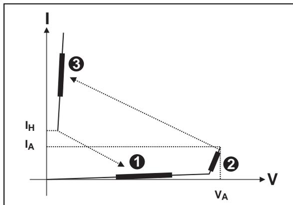
The arrows indicate the way the device is activated from point ❷ to point ❸, and the way it goes back in idle state, point ❸ to point ❶
