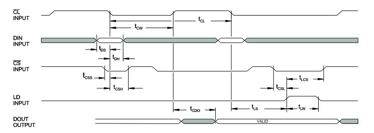
Figure 5. TIMING DIAGRAM
