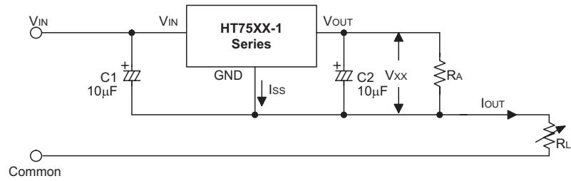
$$I_{OUT} = \frac{V_{XX}}{R_A} + I_{SS}$$
