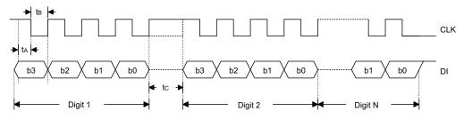
• Data latch timing for 5-bit pattern (MODE=1)
