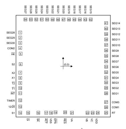
$\label{eq:Chip size: 128 x 141 (mil)} Chip size: 128 \times 141 \ (mil)^2$  \* The IC substrate should be connected to VDD in the PCB layout artwork.
