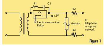
and C1 debouncing circuitry is required. Additionally, there are two fusible resistors, R2 and R3, in series with the tip and ring lines that are required for this circuitry to pass the FCC Part 68 lightning surge test. Without these resistors the relay would almost certainly be destroyed due to contact welding during such a surge.
