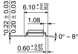
\*Dimension including the plating thickness
