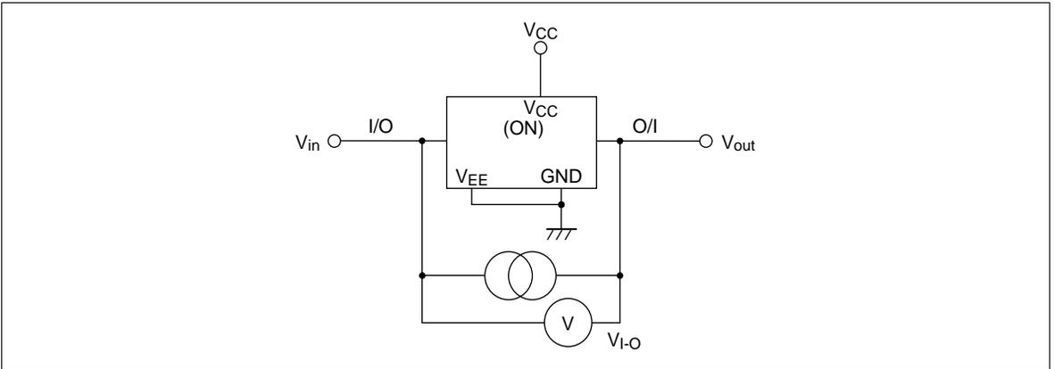
**I<sub>s</sub> (OFF): OFF Channel Leakage Current (Switch OFF)**
