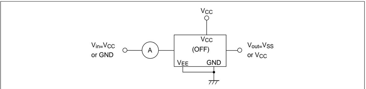
**I<sub>s</sub> (ON): ON Channel Leakage Current (Switch ON)**
