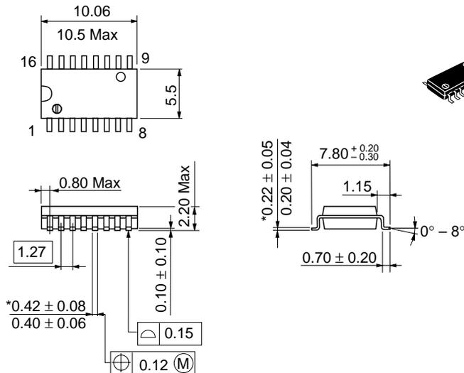
\*Dimension including the plating thickness
