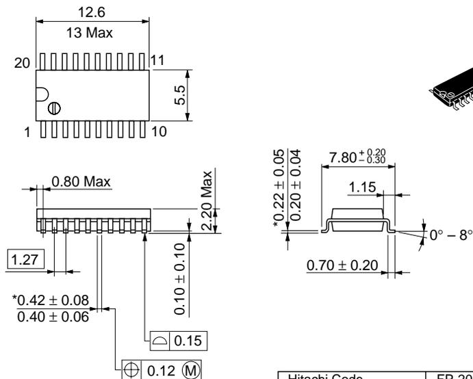
\*Dimension including the plating thickness
