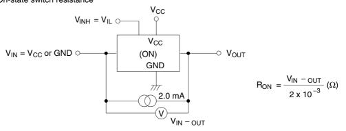
Is (OFF): Off-state switch leakage current, Is (ON): On-state switch leakage current.
