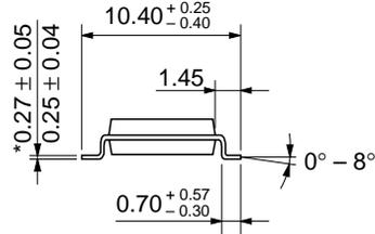
\*Dimension including the plating thickness
