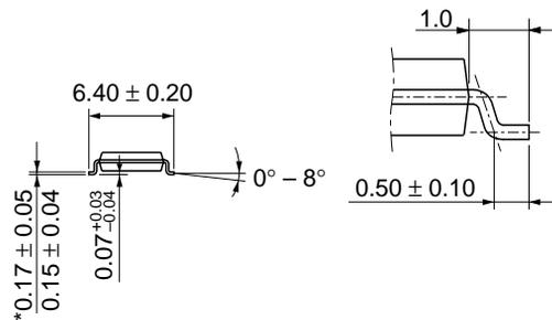
\*Dimension including the plating thickness
