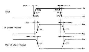
Input pulse:  $t_{TLH} \le 15 \text{ns}$ ,  $t_{THL} \le 6 \text{ns}$ , PRR = 1 MHz, duty cycle 50%.
