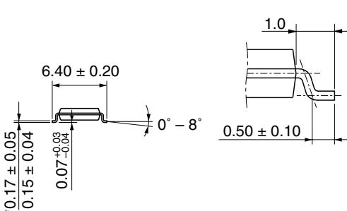
\*Dimension including the plating thickness
